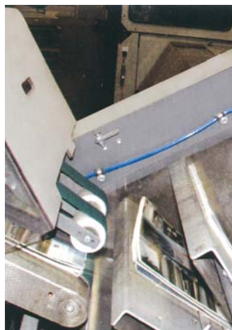
▲ Feeding of the perfect binder takes place after separation.
